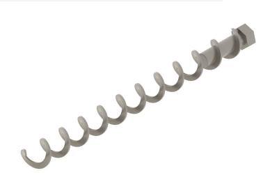
**Full screw (with center rod)** - solution preferred for well-flowing material with high bulk density (above 1,200 [kg/m3]) and highly abrasive material. Center rod reduces the risk of uncontrollable flow occurrence. Additionally, it is possible to apply **bearings on both ends** of feeding tool.
