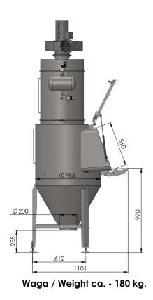
Note: the dimensions of the station may vary depending on the selected device for the further transport of bulk material.
